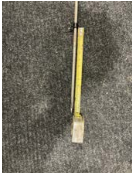
Non Treated End of Year with moisture in the ground. 12.5" depth to 200 lbs resistance
